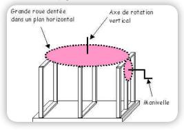
Large cogged wheel vertical rotation axis on horizontal plane
